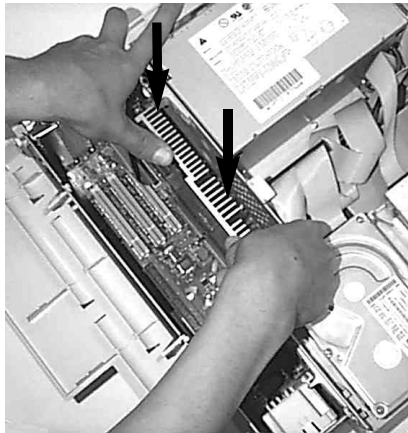
Picture 8 Installation of the MACCELERATE!750 accelerator board
